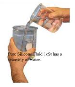
**PSF-1cSt Pure Silicone Fluid** is a 100% linear Polydimethylsiloxane composed mainly of Octamethyltrisiloxane (CAS#107-51-7) with a viscosity of 1cSt @ 25°C. The fluid is clear, colorless and essentially odorless.
