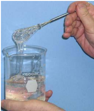
Pure Silicone 100,000cSt is a high viscosity PDMS silicone that meets VV-D-1078 "Silicone as Damping Fluid"
